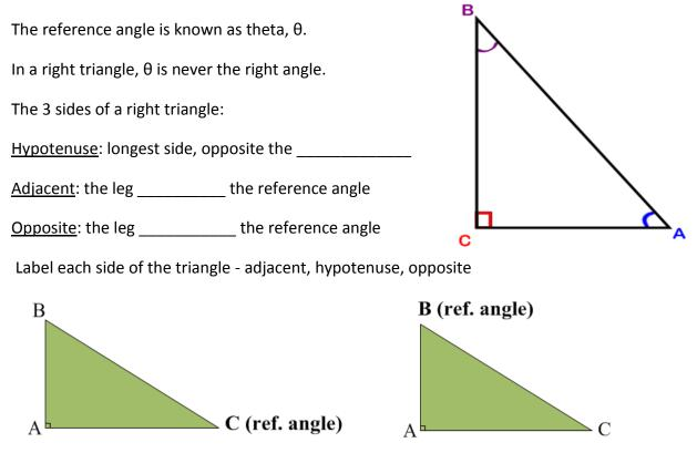
A <u>trig ratio</u> shows a relationship between two sides of a right triangle and a related angle. An easy way to remember trig ratios is: SOH CAH TOA
